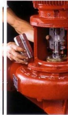
2) Remove the coupling from the pump. The coupling halves (with drive and annular positioning keys) are taken from motor and pump shafts. Loosen set screws on seal rotating element and slide from pump shaft. (For inside seal see step (3))
