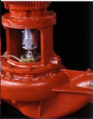
coupling with outside seal. Axially removed. Coupling bolts are still in place. Rotating element of seal is seen below the coupling, above gland plate.
